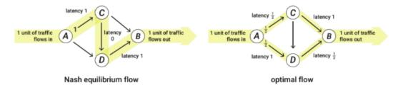
A Nash equilibrium flow has all of the traffic travel to C, then to D, and then to B. This has a latency of 2 for every driver, as opposed to the optimal form from before, which only had a latency of 3/2 for each driver. So adding edges is not always efficient.
